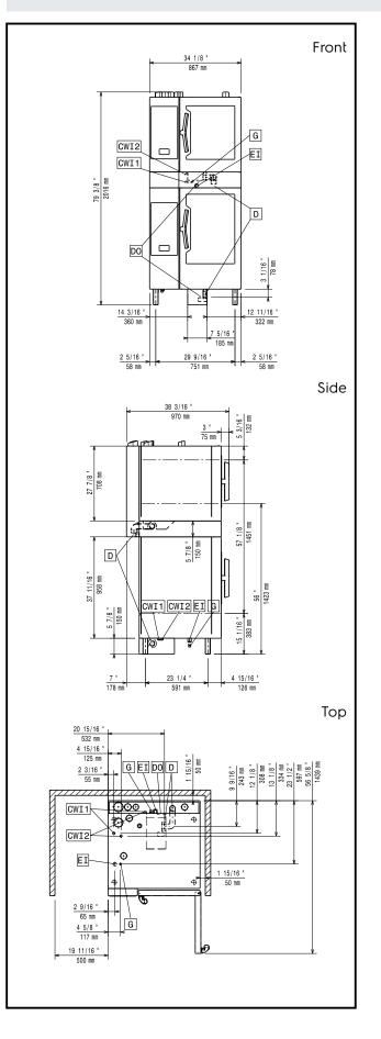
Installation accessories Stacking kit for 6 GN 1/1 oven placed on gas 10 GN 1/1
